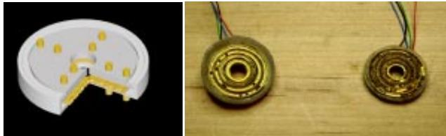
**Figure 2.** Physical view of connection mechanism (a) on the cube faces and (b) at the link ends for cable twist prevention
